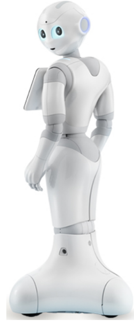
Fig. 1. Pepper is a humanoid robot standing on a holonomic mobile base, equipped with three omnidirectional wheels. It is developed by Aldebaran Robotics for the Japanese Telecommunication Company Soft Bank, to welcome customers in their shops.
