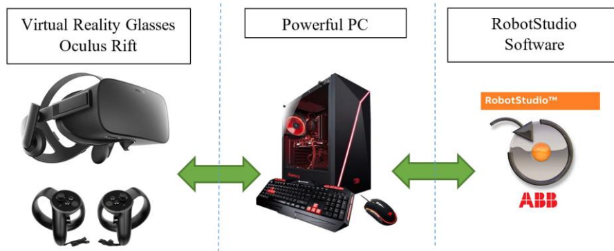
Fig. 4. The concept of cooperation of RobotStudio software with VR tools.
