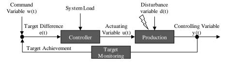
Fig. 1. Closed-loop production control [according to 11]
