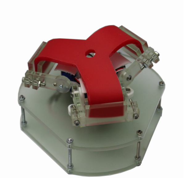
Fig. 7: The Tripod Robot is composed of a soft silicone piece actuated by three servomotors, the robot can achieve a nearly infinite number of shape configurations.
