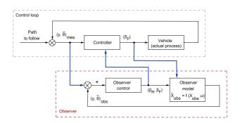
Fig. 9. Observer principle scheme
