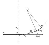
Fig. 4. Connection with an arc of clothoid
