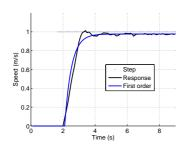
Fig. 11. Longitudinal step response: identification with  $1^{st}$  order
