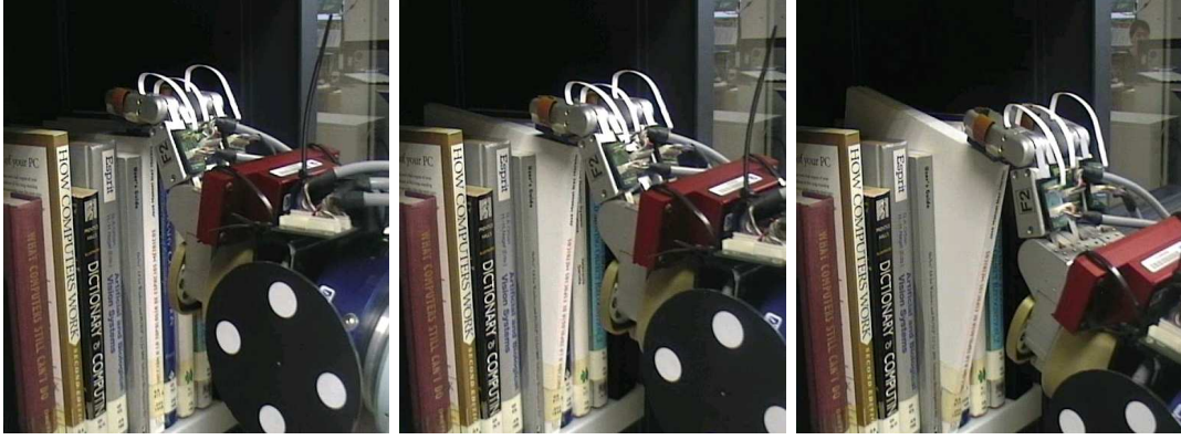
Fig. 3. The robot grasping the book by means of force and tactile-based continuous estimation of hand-to-object relative pose.
