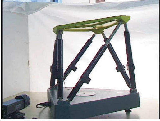
Fig. 3. Experimental set-up: A Gough–Stewart platform observed by a camera.
