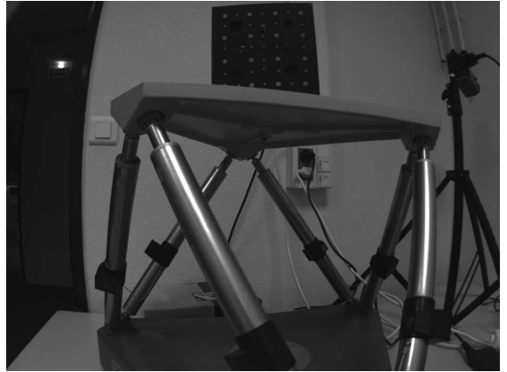
Figure 1: A Gough-Stewart platform observed by a camera with short focal length.
