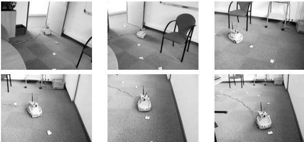
Fig. 5. Following a visual route: the previously learnt visual path, about 10m long, is materialized on the ground. The pictures were taken during an autonomous run
