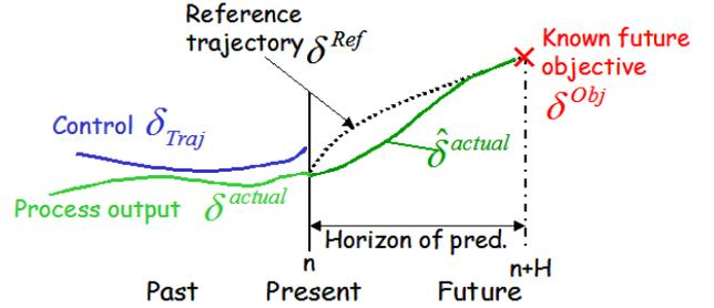
Fig. 4. Notations and general description of MPC
