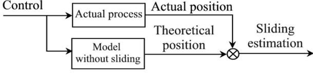
Fig. 3. Sliding detection
