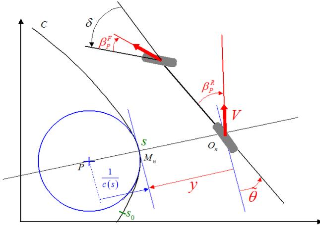
Fig. 1. Classical kinematic model parameters
