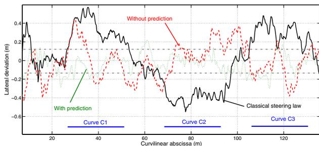
Fig. 10. Lateral deviation during path #2 following
