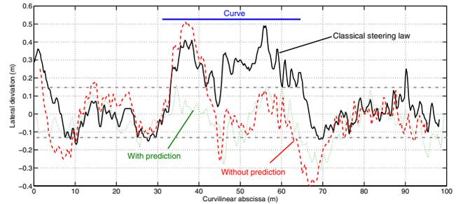
Fig. 9. Lateral deviation during path #1 following
