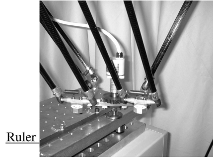
Fig. 5 : Validation experiment - Kinematic constraint on the end-effector
