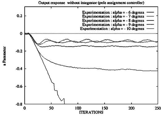
Figure 15.  $a$  with perturbations ( $\alpha = -6$  to  $-10$ ) (experimental results).
