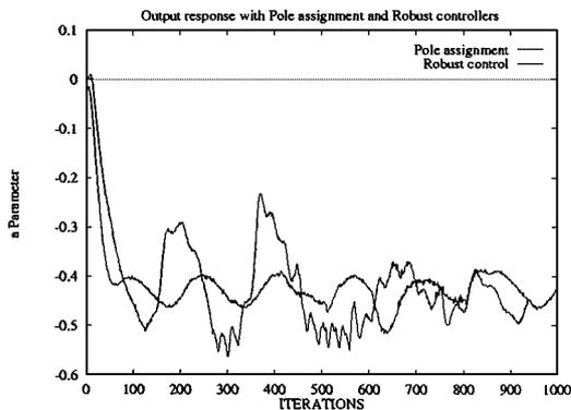
Figure 33. Parameter  $a$  (robust and pole assignment control) (experimental results).
