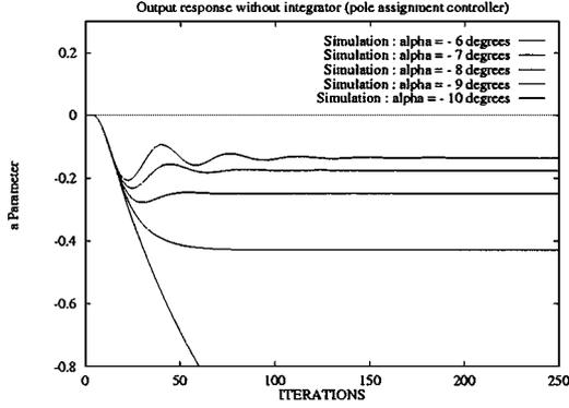
Figure 14.  $a$  with perturbations ( $\alpha = -6$  to  $-10$ ) (simulation results).
