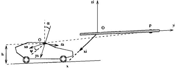
Figure 3. Perspective projection of a 3D line.
