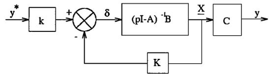
Figure 4. Visual servoing scheme with a pole assignment.
