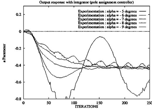
Figure 17.  $a$  with perturbations ( $\alpha = -5$  to  $-9$ ) (experimental results).
