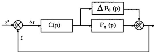
Figure 18. Servoing scheme in  $H_\infty$  space.
