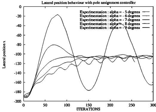
Figure 24. Lateral position behavior (pole assignment) (experimental results).
