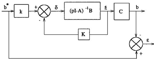
Figure 9. Steady state error.
