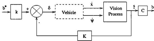
Figure 5. Visual servoing scheme of the simulator.
