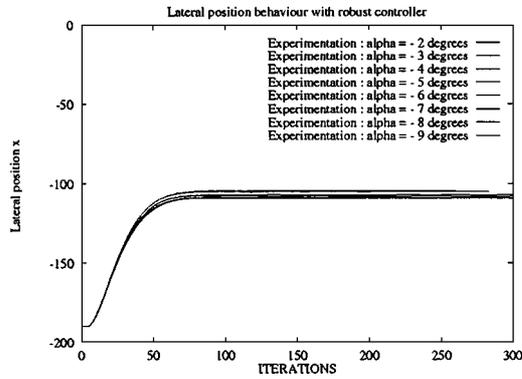
Figure 25. Lateral position behavior (robust control) (experimental results).
