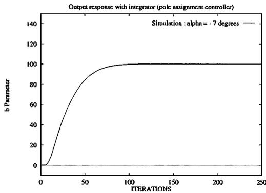
Figure 11.  $b$  without perturbations ( $\alpha = -7$ ) (simulation results).
