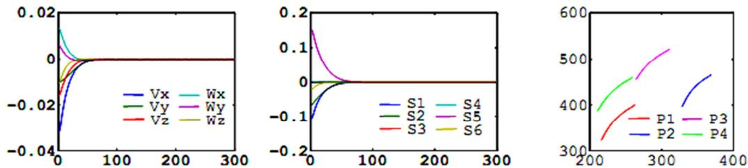
Fig.6. ER1 using  $s_\lambda$ . Left: camera velocity (in m/s and rad/s), middle: visual features errors, right: image points trajectories.
