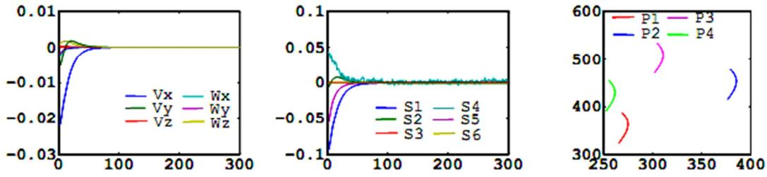
Fig.7. ER1  $s_m$ . Left: camera velocity (in m/s and rad/s), middle: visual features errors, right: image points trajectories.
