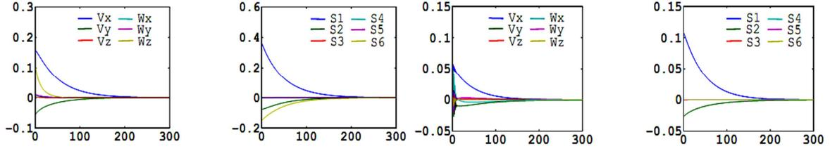
Figure.4. Simulation results with non-symmetrical image using  $s_\lambda$ . Left: camera velocity (in m/s and rad/s); right: visual features errors.
