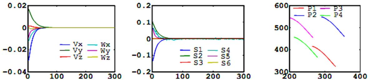
Fig.9. ER2  $s_m$ . Left: camera velocity (in m/s and rad/s), middle: visual features errors, right: image points trajectories.
