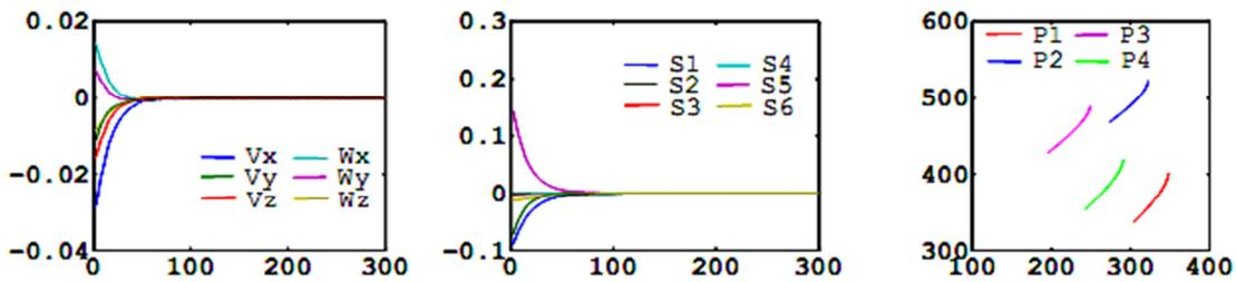
Fig.8. ER2  $s_x$ . Left: camera velocity components (in m/s and rad/s), middle: visual features errors, right: image points trajectories.
