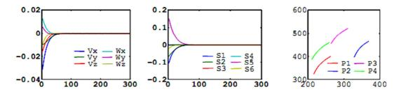
Fig.6. ER1 using  $s_{\lambda}$ . Left: camera velocity (in m/s and rad/s), middle: visual features errors, right: image points trajectories.
