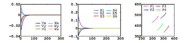
Fig.8. ER2  $s_{\lambda}$ . Left: camera velocity components (in m/s and rad/s), middle: visual features errors, right: image points trajectories.
