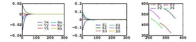
Fig.9. ER2 s<sub>m</sub>. Left: camera velocity (in m/s and rad/s), middle: visual features errors, right: image points trajectories.
