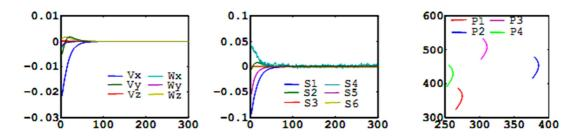
Fig.7. ER1 s<sub>m</sub>. Left: camera velocity (in m/s and rad/s), middle: visual features errors, right: image points trajectories.
