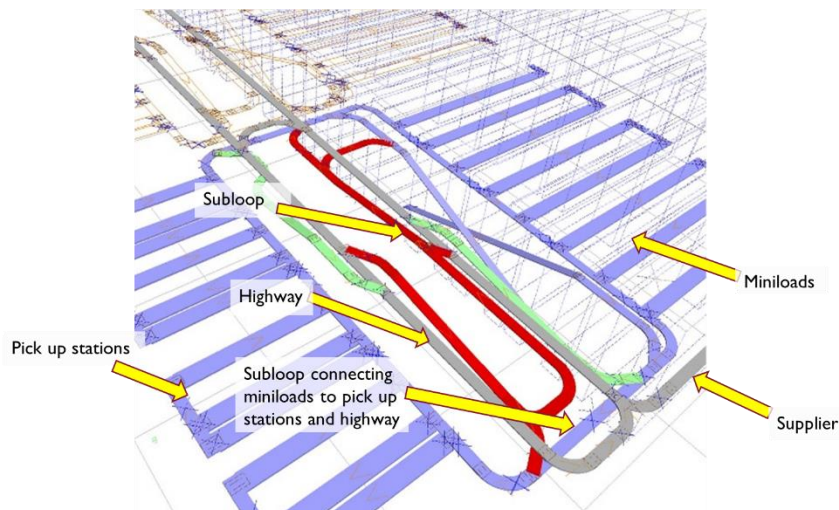
Fig. 1. The geometry of the modular conveyor system under study (Courtesy of ASKO and Swisslog).
