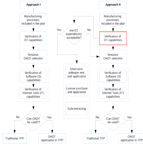
Fig. 3. The approaches of OADT application in TPP of SMMEs.
