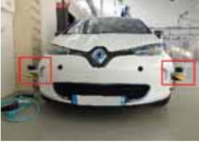
Sick LMS151 installed on the front
