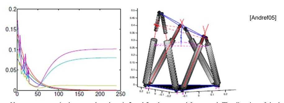
Non-convergence in the case where legs 1, 2 and 3 only are used for control. The direction of the legs are superimposed (red) on the cylinders. A leg has converged to its desired orientation if its direction crosses the endeffector in the desired pose at the joint location. Notice that this happens only for the 3 controlled legs.
