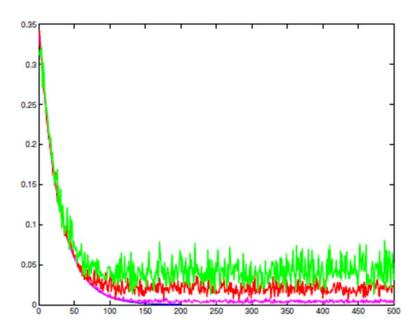
Robustness to noise: sum of squares of the errors E<sup>T</sup>E *vs* time with a noise amplitude of 0.01 deg (dashed), 0.05 deg (dashed) and 0.1 deg (dash-dotted).
