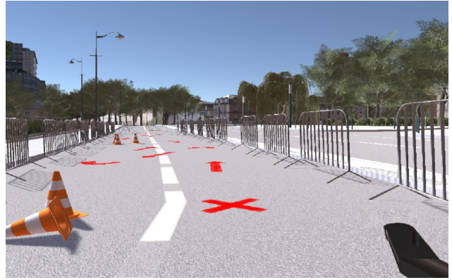
Figure 3: Participant point-of-view during trials. The black part in the bottom-right corner corresponds to the arm of a virtual wheelchair, which is spatially collocated with the real joystick and vestibular feedback platform.
