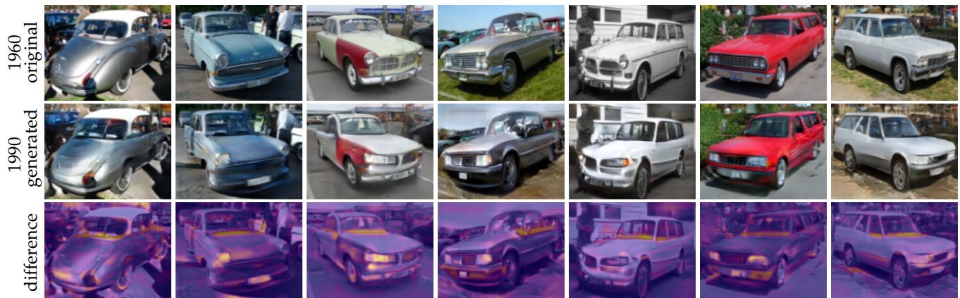
(a) Input images of cars from the 1960s (top row) and their generated translations into 1990s (middle row). The difference images (bottom row) highlight the changes in the headlights of the cars, going from small round ones to large rectangular ones, as well as the increasing size of the car windows and windshield.
