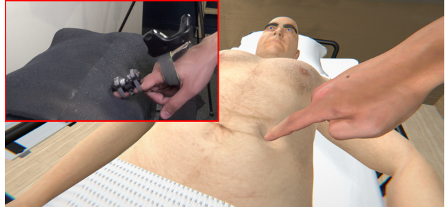
Fig. 1. Application example. A human user wearing a finger device interacts with a tangible object that resembles the abdomen of a virtual human patient. Providing timely cutaneous stimuli via the wearable haptic device, we can alter the stiffness and shape perception of passive tangible objects. For example, in the context of medical palpation, we can simulate the presence of a tender body part or of a small bump representing a cyst.
