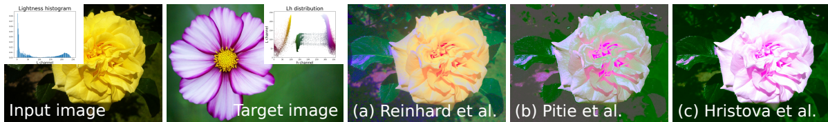
Figure 1: Results (a) and (b) are obtained using two global color transfer methods (Reinhard et al., 2001; Pitié and Kokaram, 2006). The input image consists of two lightness clusters (corresponding to the two main peaks in its lightness histogram), whereas the target image is composed of three color clusters (as shown in its lightness-hue plot). Due to this fact, the global color transformations fail to produce plausible results. Result (a) does not match the target colors, whereas result (b) is significantly over-saturated, which compromises its photo-realism. Result (c) is obtained using a local color transfer (Hristova et al., 2015), which increases significantly the quality of the color transfer and the result.
