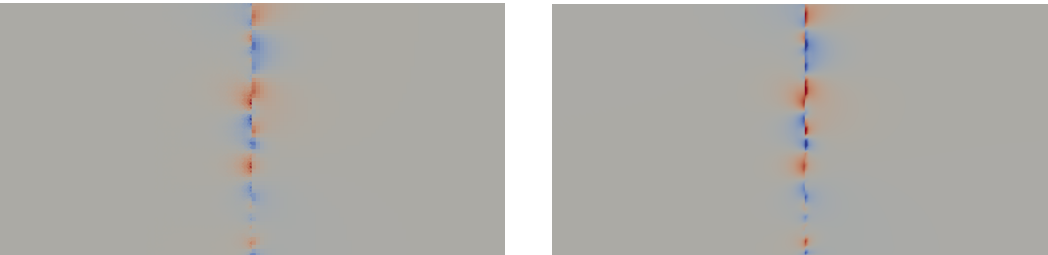
Fig. 10 Error \mathbf{u}_x^{10} - \mathbf{u}_x at the 10 th iteration. Left: Primal mesh, \|\mathbf{u}_{\mathcal{M}}^2 - \mathbf{u}_{\mathcal{M}}\|_\infty = 0.52 . Right: Dual mesh, \|\mathbf{u}_{\mathcal{M}^* \cup \partial\mathcal{M}^*}^2 - \mathbf{u}_{\mathcal{M}^* \cup \partial\mathcal{M}^*}\|_\infty = 0.05 .
