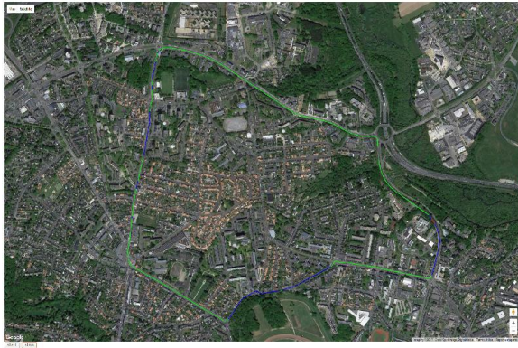
Fig. 9. RTK-GPS coverage - Urban zone (RTK zones in green)
