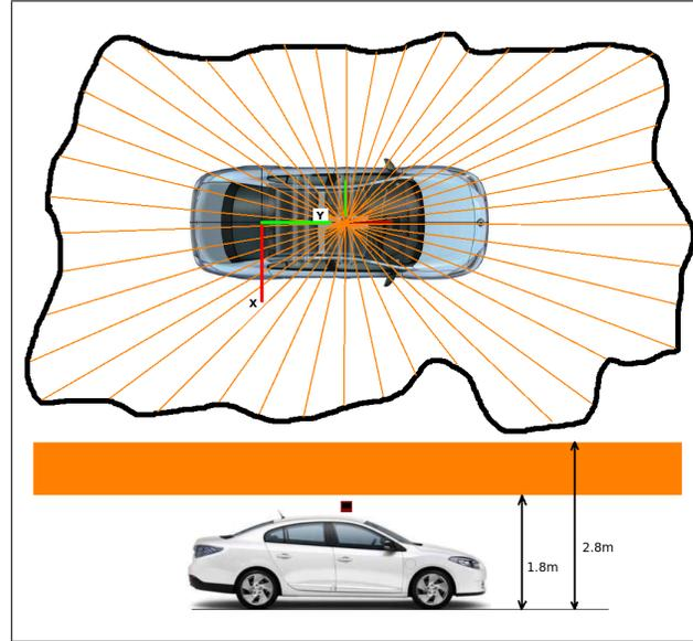
Fig. 3. Sensor configuration for Fluence. A  $360^\circ$  laser scan is obtained from the 3D point-cloud generated by the VLP-16. The bottom of the figure shows the point-cloud range involved in the generation of the planar scan.
