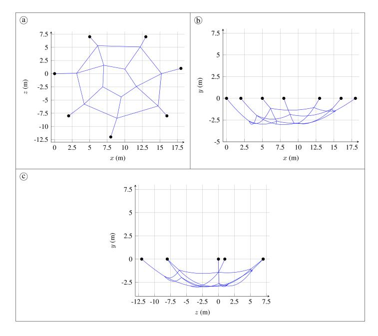
Figure 13: Rest configuration of a cable net structure (solid line —) under three different views - (•) for clamped cable end (4803 dofs and 120 bilaterals constraints)
