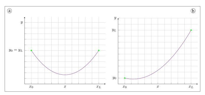
Figure 5: Rest configuration of an aligned cable (a) (FEM error =  $1e^{-5}$ ) and inclined cable (b) (FEM error =  $7e^{-8}$ ) obtained via FEM (solid line —) and obtained analytically (dashed line ---)
