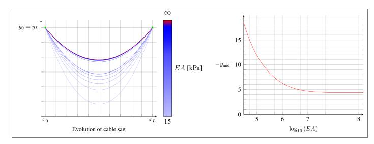
Figure 6: Rest configuration of a cable with respect to the case 1 obtained by FEM with rigidity EA varying from 1 kPA to 1 GPA (left); Evolution of mid-span deflection with the logarithm of cable rigidity,  $\log (EA)$  (right)
