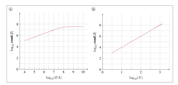
Figure 12: Evolution of the conditioning  $(\log_{10})$  of the Jacobian matrix with regard to (a) the weight/rigidity ratio and with regard to (b) the number of elements
