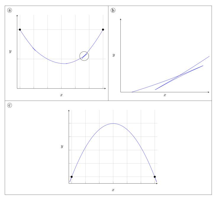
Figure 1: Results obtained from standard FEM modelling of the cable: ⓐ creation of a loop; ⓑ zoom at one loop of ⓐ; ⓒ creation of compression and folds for a cable (solid line —) with end nodes imposed (•)
