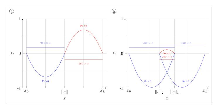
Figure 2: Analytically obtained profiles of a cable with corresponding dilatation where the positiveness of  $\varepsilon$  is removed from assumptions. Cable may exhibit tensed segments (solid line —) or compressed segments (solid line —)
