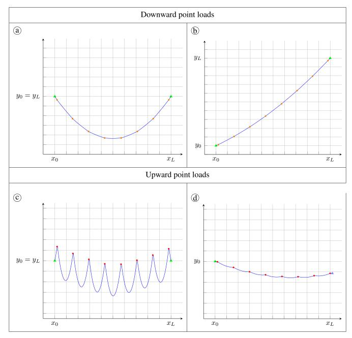
Figure 7: (a) Cable at rest (solid line —) subjected to downwards point loads at given positions (•) for aligned and
