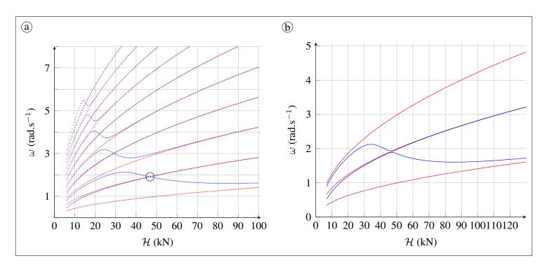
Figure 16: Evolution of the first frequencies of the system with regards to the horizontal tension obtained from (a) analytic method [2] and (b) numerical method
