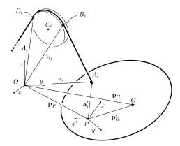
Fig. 1: Geometry of the cable-driven robot
