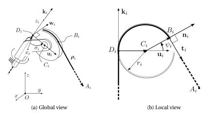
Fig. 2: Geometry of the swivel pulley
