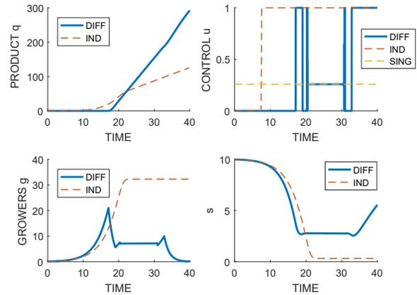
Fig. 4. **Chemostat mode, 40 hours.** Optimal solutions for induction and differentiation systems. The value of  $u$  on a singular arc in steady state is superposed to the graph. Since the control value cannot be deduced from the expression of  $\dot{H}_u$  over a singular arc, we may expect a chattering phenomenon of the control at junctions with singular arcs of Fuller type [4]. And this is indeed what we observe.
