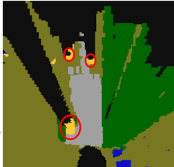
Bird's Eye View Ground-Truth => Frontal View GT projected using Point-Clouds (Bayesian Perception) => Densified by humans (different resolutions of images & point-clouds)
