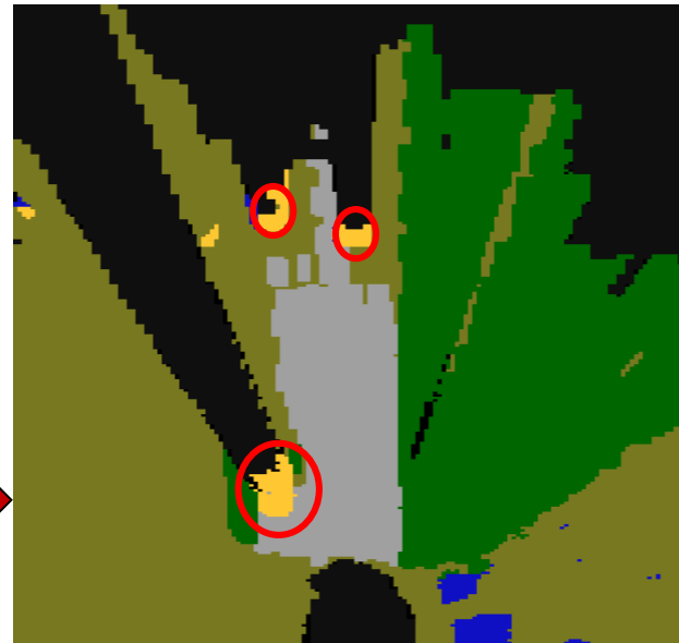
Bird's Eye View Ground-Truth => Frontal View GT "projected" using Point-Cloud (Bayesian Perception) => Densified by humans (point-clouds and images have different resolutions)
