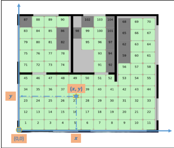
Fig. 4. The position coordinates of a person in the global frame of the platform plan represented on the cartography of the tiles with their identifiers. Note that, the red dots in the corners of tiles indicate the positions of the load pressure sensors.
