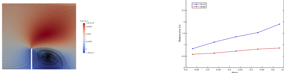
Figure 1: Vertical plate in a flow at \text{Kn} = 0.0345 . Streamlines and horizontal velocity component (left panel). Prediction error (right panel). The database is created for a Mach number of 0.63 and the predicted solutions are for Mach 0.23,0.33,0.43,0.53,0.63. The number of modes is either 15 or 20. Computational time is divided by 45.
