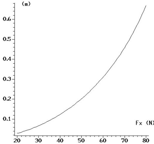
Figure 3: Difference in meter between the cable length and the distance between the attachment points  $A, B$  as function for  $F_x$  (N) for a total tension of 100N and a cable length at rest of 50 meters. This figure clearly shows that the sagging effect induces a large difference between the measured cable length and the distance between  $A, B$  as soon as  $F_x$  increases.
