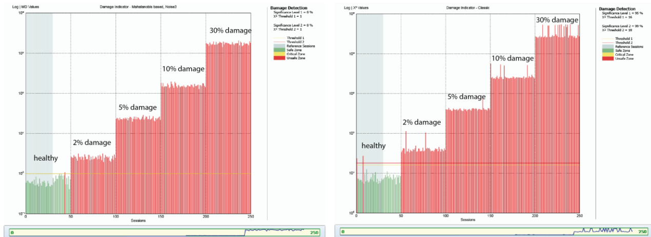
Figure 4. Damage detection in simple system. Case-3% of noise in the response. Damage indicators for the Mahalanobis-based (left) and robust subspace-based (right).
