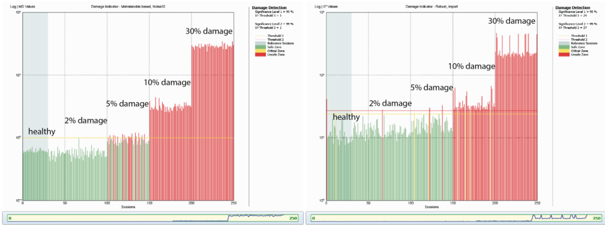
Figure 5. Damage detection in simple system. Case-30% of noise in the response. Damage indicators for the Mahalanobis-based (left) and robust subspace-based (right).
