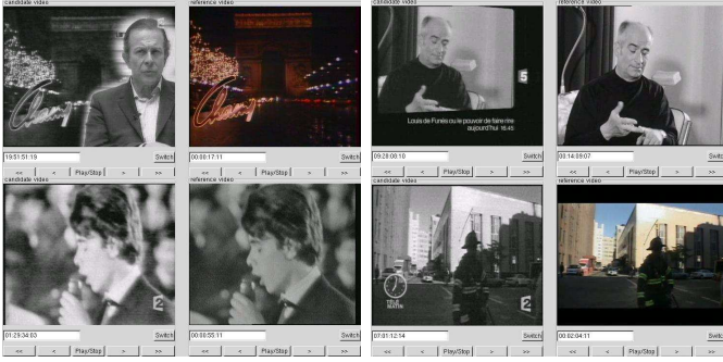
Fig. 18. Four good detections of the TV monitoring system: the left image of each match is the broadcasted video (captured in black and white) and the right image of each match is the retrieved video
