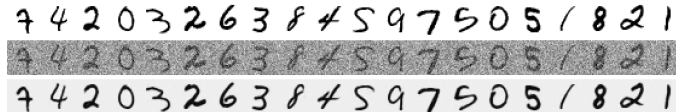
Figure 3: ( \sigma \approx \sigma_c ) Denoising performance of DEEN with a single jump for \sigma = 0.3 . The noisy pixel values are in the range [-1.200, 1.995] , and the denoised ones are in [-0.0749, 1.0539] .
