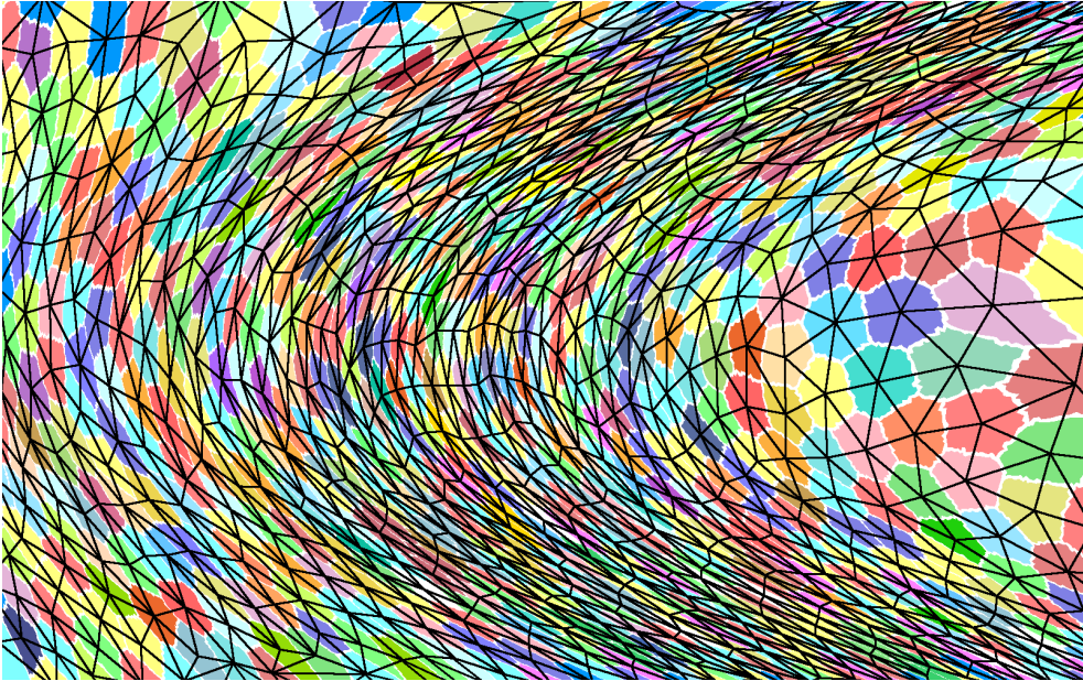
FIG. 1. The discrete Riemannian Voronoi diagram (colored cells with bisectors in white) and its dual complex (in black) realized with straight simplices of a two-dimensional domain endowed with a hyperbolic shock-based metric field.
