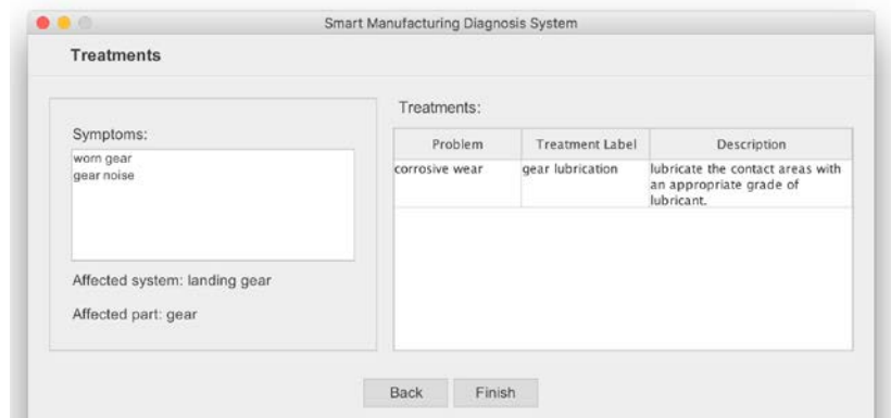
Fig. 5. SMDS tool screenshot (4): the tool suggests the treatments based on the selected root causes
