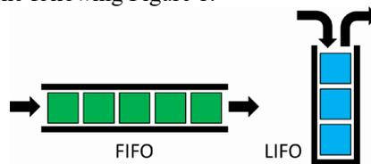
Figure 1: Simplified illustration of FIFO and LIFO
