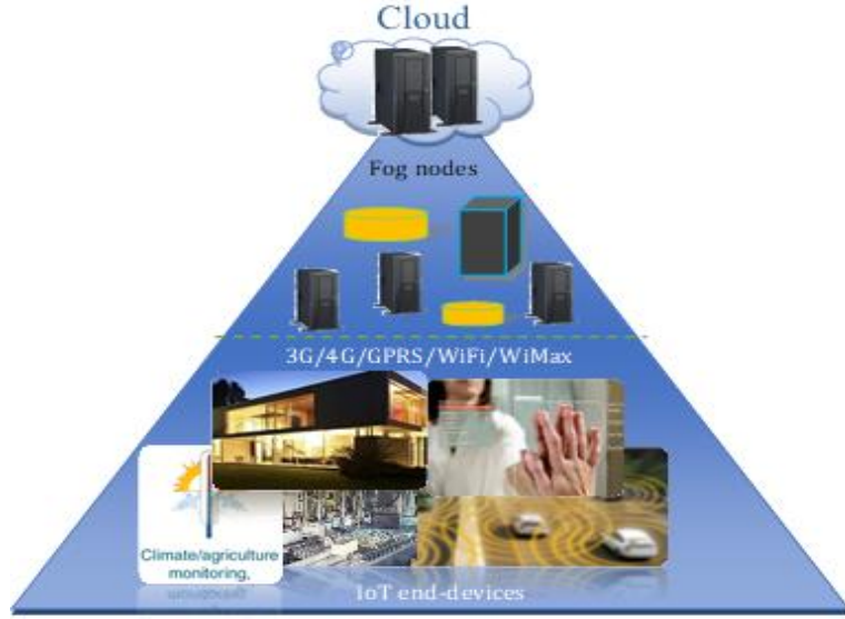
Fig. 1. IoT ecosystem comprising three layers: cloud, fog, and end-device layer [2]
