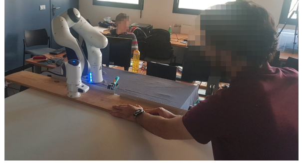
Fig. 5: Experimental mock-up including a table, a guiding rail, a wooden board, the Panda robot and one of the three subjects. The pulley system and load used to produce the emulated cutting force are placed under the table.
