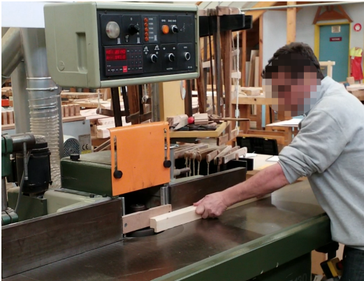
Fig. 1: Illustration of a wood milling task by a trained expert on a wood shaper. The left arm maintains lateral stability while the right arm (hidden on this picture) pushes the part in direction of the cutting tool.
