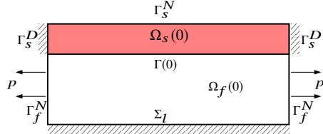
**Fig. 3** Geometrical configuration for the FSI-contact model. We apply a porous medium model on the (rigid) lower wall, where contact might take place.
