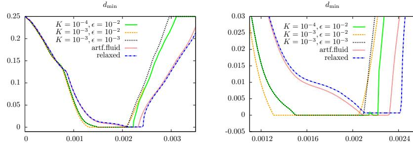
**Fig. 4** Minimal distance of  $\Omega_s$  to the lower wall  $\Sigma_p$  over time. Right: zoom-in around the contact interval. We compare the new approach presented in Section 3 for different parameters with the *artificial fluid* and the *relaxed* contact approach studied in [4].
