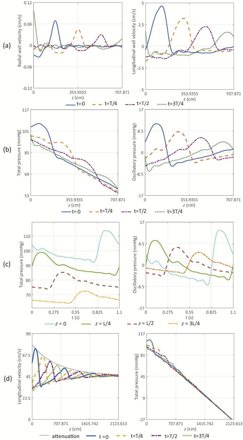
**Figure 3.**(a) Radial and longitudinal velocity along the vessel wall at different times  $mT/4$ ,  $m = 0, \dots, 3$ ; (b) Total and oscillatory pressures along the vessel at different times; (c) Total and oscillatory pressure versus time at different cross sections of the vessel  $z = m\lambda_1/4$ ,  $m = 0, \dots, 3$ ; (d) Total centerline velocity and pressure at different times of the cardiac cycle over three spatial wavelengths  $L = 3\lambda_1$ .
