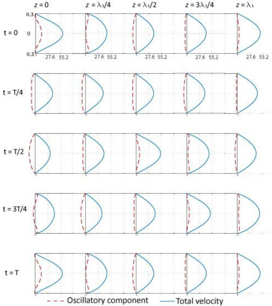
**Figure 2.** Longitudinal velocity profiles along the vessel: periodicity in time with period  $T$ ; periodicity in space with period  $\lambda_1$  and attenuation in the oscillatory component are observed.
