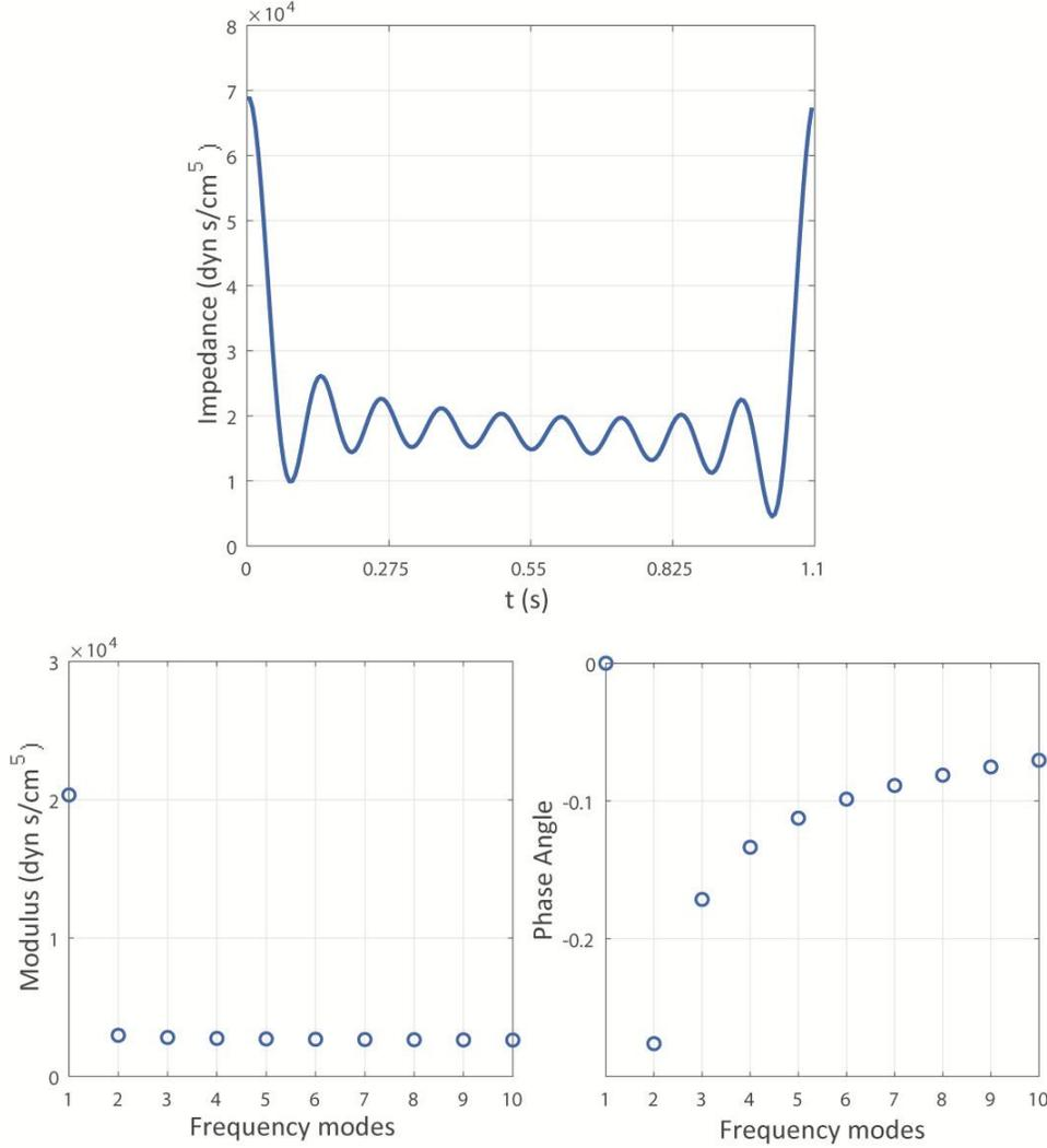
**Figure 5.** Impedance function  $z(t)$  in time domain at  $z = L = 12.6$  cm. Inserts depict the 10-mode reconstruction of the modulus and phase of the impedance function in the frequency domain  $Z_n$ .
