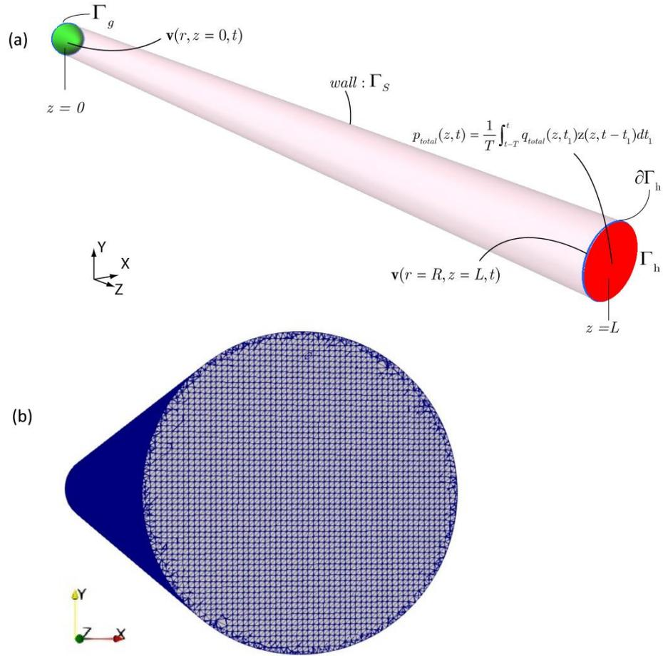
**Figure 4.** (a) Inlet and outflow boundary conditions prescribed in the numerical domain: straight cylinder with a length  $L = 12.6$  cm ; (b) Cut plane through the central section of the vessel ( $z = 6.3$  cm), showing the structured nature of the mesh in the interior of the vessel.
