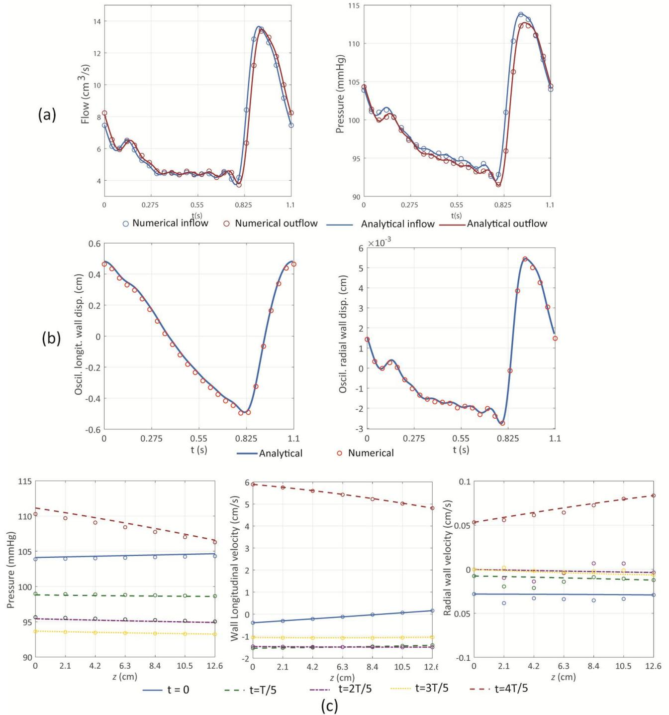
**Figure 6.** (a) Numerical versus analytical solution: flow and pressure at inlet and the outlet of the vessel; (b) Oscillatory parts of wall longitudinal and radial displacements over time, at  $z = L/2 = 6.3$ ; (c) Comparison between the analytical (lines) and numerical (circles) wall pressure (left), wall longitudinal velocity (middle), and radial velocity (right) along the vessel axis at different times.
