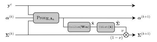
Figure 3: An illustration of one step of the main inference algorithm for GroupSC.
