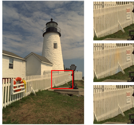
Figure 2: Demosaicking result obtained by our method. Top right: Ground truth. Middle: Image demosaicked with our sparse coding baseline without non-local prior. Bottom: demosaicking with sparse coding and non-local prior. The reconstruction does not exhibit any artefact on this image which is notoriously difficult for demosaicking.
