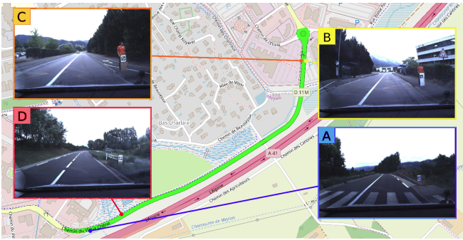
Fig. 6: Snapshot of OpenStreetMap illustrating the test route and respective positions of AprilTag markers.
