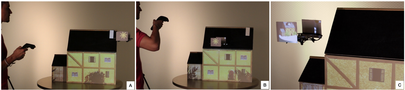
Figure 4: (A - B) The light source of our scene is at the drone hovering position. By moving the light source, the user is casting shadows on the scene. (C) An interactive 3D model of the mock-up displayed next to the physical one allows the user to observe the scene from another viewpoint.
