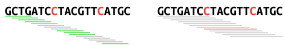
Fig. 2. Patterns of weak k -mers resulting from a sequencing error, depending on k . Sequencing errors in the read are pictured in red. Solid and weak k -mers are represented respectively with green and grey lines, with k = 4 (left) and k = 8 (right). The k -mer pictured in red contain two errors. A sequencing error usually impacts k k -mers and creates a weak region of size 2 * k - 1 (left). Choosing a large k results in most k -mers of a read being weak as they contain one or several errors (right).
