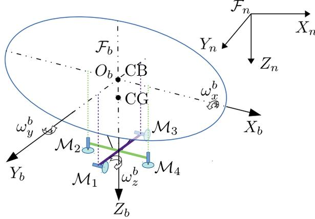
Figure 1: Reference frames for indoor blimp robot
