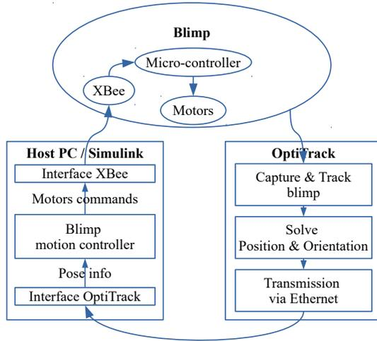
Figure 11: Scheme of Optitrack-enhanced blimp control system
