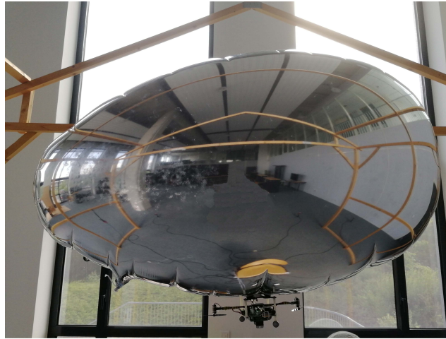
Figure 10: The blimp robot studied in this work
