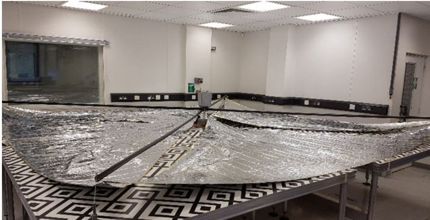
Figure 28. Ground testing of the dragsail for the SSO-A mission.
